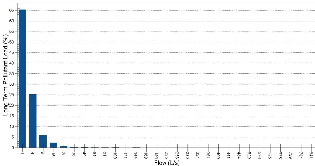
**Figure 2. Long Term Pollutant Load by Flow Rate for TORONTO CENTRAL – 100, 1982 to 1999 for 0.3 ha, 90% impervious.** The majority of the annual pollutant load is transported by small frequent storm events. Conversely, large infrequent events carry an insignificant percentage of the total annual pollutant load.
